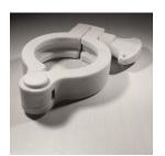
Sanitary Non-metallic Clamps designed as alternative to Standard Stainless-Steel Clamp. These are often used in single-use disposable applications. They are manufactured using a glass-reinforced, FDA grade, USP Class VI Nylon. Usually used in lower pressure 150 psi or udder applications. Developed for use in both non-metallic and metallic connections. Also, the clamps generally won't damage or distort non-metallic ferrules. In addition, they are very light weight.
